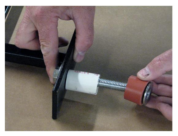
Screw the rubber expansion fastener on the bolt.
