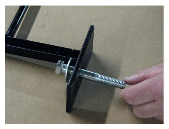
Insert bolt with washer through the mounting plate.
