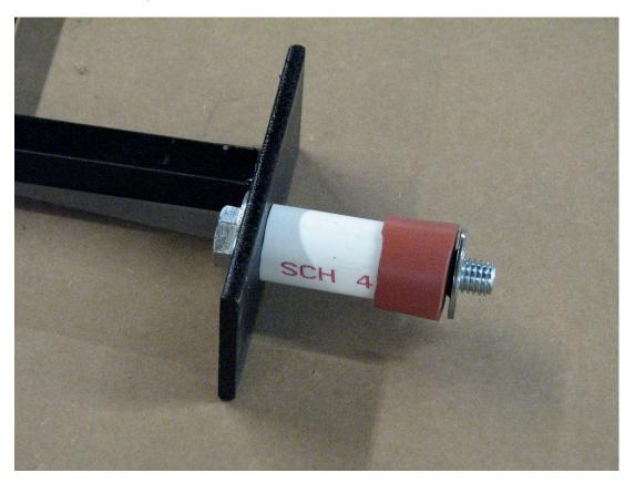
Continue threading the expansion fastener onto the bolt until it touches the PVC spacer. Set the rack onto the bed of your Ranger aligning the bolting holes of the bed to the bolt. Press down to insert the rack into the bolt holes. Lightly tighten the bolt to expand the rubber fastener which locks the rack onto the bed. DO NOT OVER TIGHTEN THE MOUNTING BOLT!
