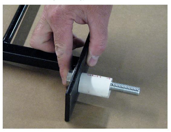
Slide PVC spacer onto the bolt.
