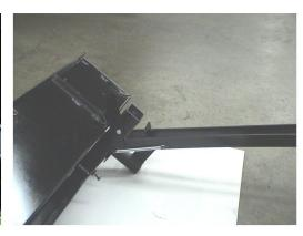
Attach handle using 5/16 x 3" bolt and nut. Install spring in the shown position.
