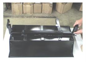
Slide each attachment leg into the support frame and tighten the 2ea 1/2 x 1 1/2 bolts finger tight
