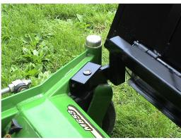
Install frame mounts onto the caster support frame of the ZTR using the supplied bolts, nuts, washers, U-brackets and backer plates
