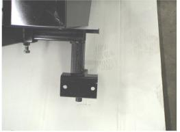
Set the assembled Quick-Dump unit into the U-brackets and secure with the supplied  $3/4 \times 3$ " pins and cotter pins. Tighten main support bolts on the bottom of the unit securely.
