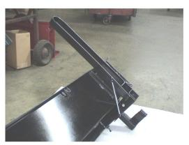
Elevate handle to the up position to lock the dump bed.
