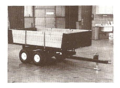
Note: If you desire to install a dump cylinder, the attachment holes are already available on the main chassis and the bed to fit a standard 24" stroke agriculture cylinder with up to a 4" diameter piston.
