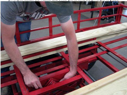
Pull the winch cable through the opening in the front of the lifting arms to the back of the lifting arms. Install the pulley on the rear lifting arm with the cable threading from the bottom of the pulley to the top. Install 1 short pivot pin to secure the pulley to the arms. Pull the cable eyelet to the front lifting arms and secure with the second pivot pin. Install the washers and cotter pins on
