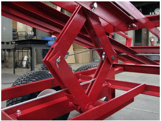
Photo shows pivot pins without washers at this point. Remove the cotter pins and install washers before installing cotter pins permanently. NOTE: CABLE ROUTING IS CRITICAL FOR CORRECT OPERATION! These 2 photos show the correct cable routing.
