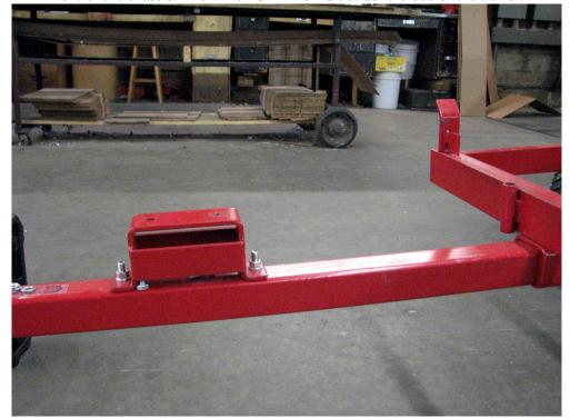
Install the lower brackets using 4 each 5/16 x 1 ¼ inch and 1 each 4 inch pivot pin. The rear of the lower lift arms has a welded end cap as shown in the photo below and must face the REAR of the trailer.
