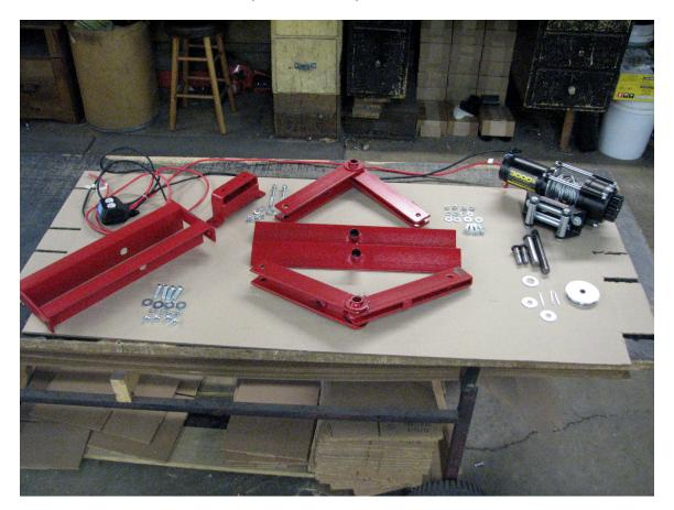
4 ft x 7 ft BEDS MANUFACTURED PRIOR TO SEPTEMBER 2020 will require drilling 4 holes in the bed frame to bolt the upper lift bracket (Trailers manufactured after Sept 2020 holes are drilled at the factory and the upper lift bracket is pre-installed if ordered with your trailer). It is easiest to install the unit with the bed removed from the chassis and the center wood boards removed from the bed of the trailer.
