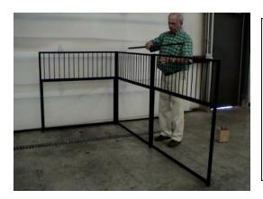
Insert a wall stiffener at the junction of the side panels. The wall stiffener replaces the need for a panel connector at the top of the side walls.
